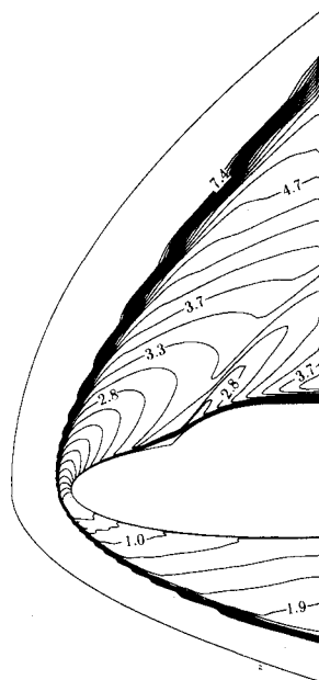
Fig. 12 Iso-Mach lines ( \Delta M = 0.25 ) for M_\infty = 8.15 , \alpha = 30 deg (RKTVD).
